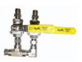
assembly. This is especially useful for injecting Hydro Gel into leaking manholes. High pressure valve. 2000 psi and under. Use with grout needle or wall stinger nozzle. Available in carbon steel and stainless steel.
