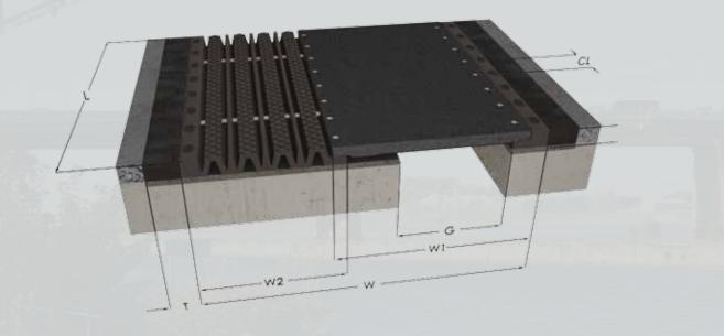
High movement Transflex modules are numbered from 1600 to 3200, and cover a movement range from 400mm to 800mm.
